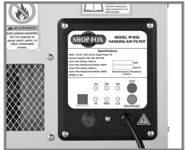
Figure 5. Air filter control panel.
