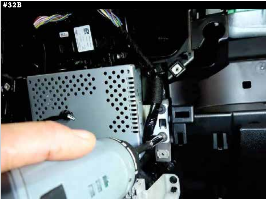
#32A 32. Remove four (4) 7mm screws securing receiver chassis, disconnect harnesses, then remove chassis.
