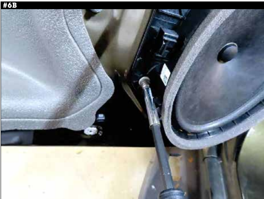
6. Remove four (4) 7mm screws securing speaker to door, disconnect harness, then remove speaker.
