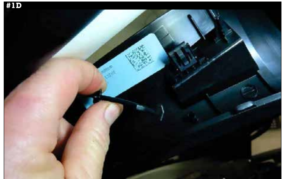
2. Twist two (2) tethers to release, then work out of slots in trim panel.
