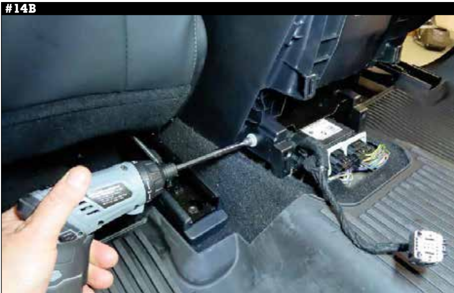
12. Remove two (2) 7mm screws exposed by removal of center console back panel.
