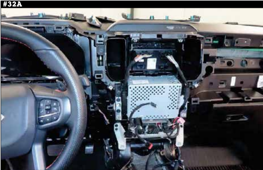
#32A 32. Remove four (4) 7mm screws securing receiver chassis, disconnect harnesses, then remove chassis.
