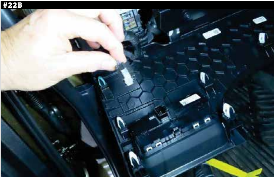
22. Pry off knee panel assembly to release two (2) clips, disconnect harness, then remove assembly.
