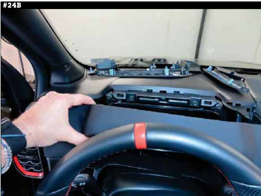
24. Pry out upper instrument cluster trim panel to release sixteen (16) clips, disconnect harness, then remove trim panel.
