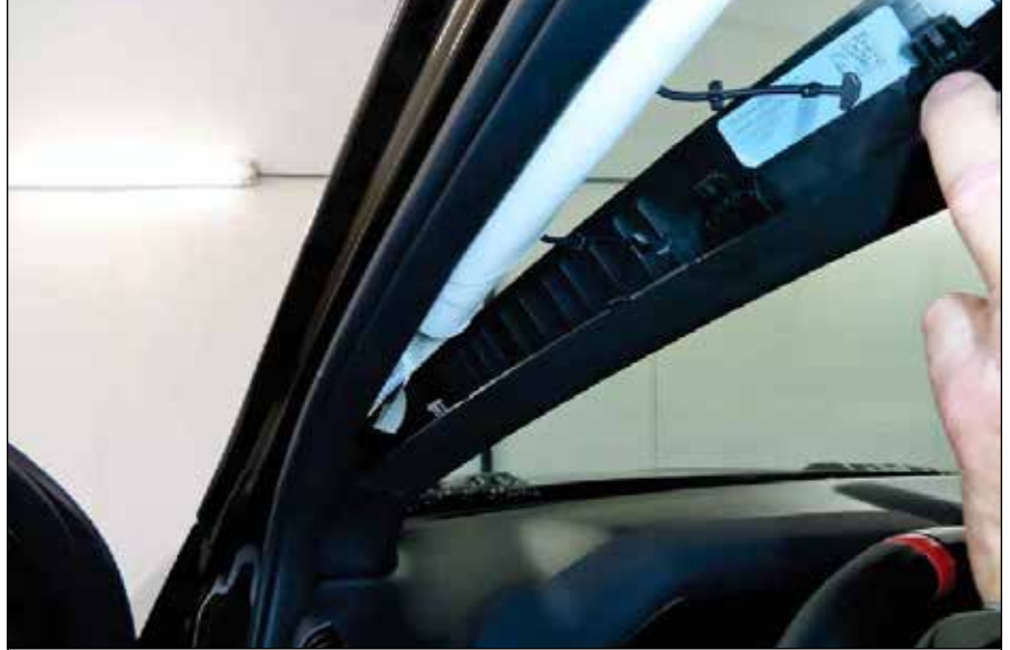
3. Lift trim panel, disconnect harness, then remove panel.
