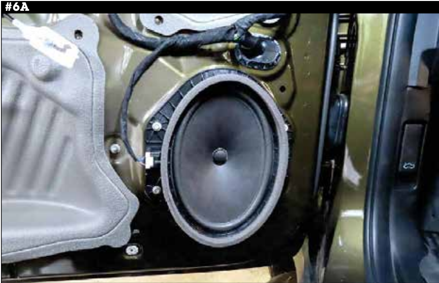
6. Remove four (4) 7mm screws securing speaker to door, disconnect harness, then remove speaker.
