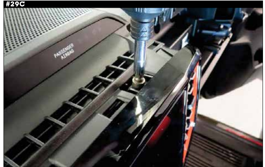
29. Remove two (2) 7mm screws exposed by removal of receiver top trim panel.
