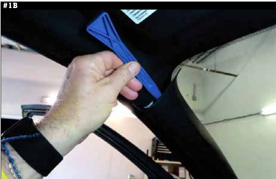
1. Starting at top edge, pry off pillar trim panel to release three (3) clips.
