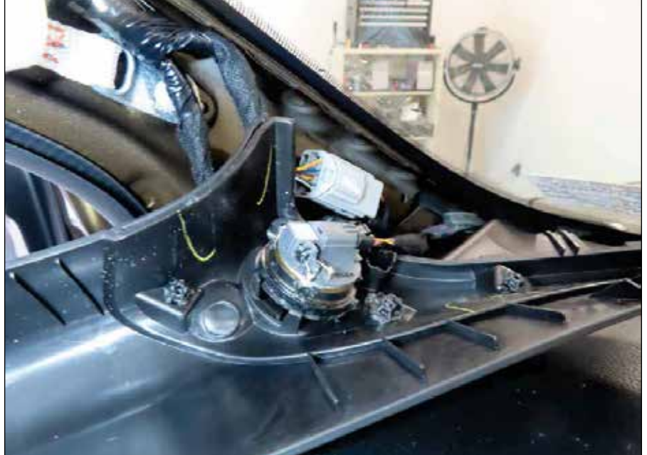
3. Lift trim panel, disconnect harness, then remove panel.
