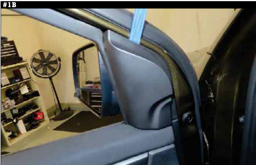
1. Starting at top corner, pry off sail panel to release three (3) clips, then remove sail panel.
