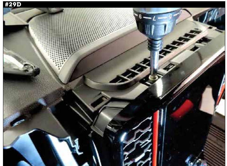
29. Remove two (2) 7mm screws exposed by removal of receiver top trim panel.
