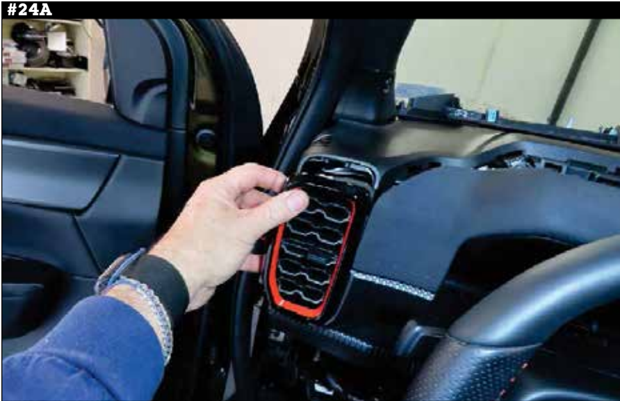
24. Pry out upper instrument cluster trim panel to release sixteen (16) clips, disconnect harness, then remove trim panel.
